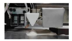
Fig. 23. Hopper mounted on the jig
