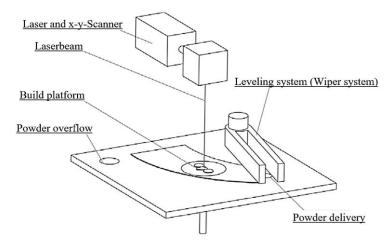
Fig. 3. Realizer 50 desktop SLM machine kinematics [11]
