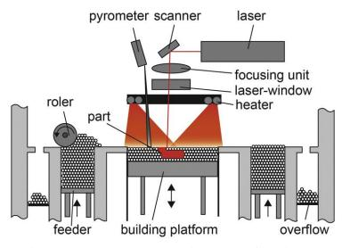
Fig. 2. Double double chamber design with overflow bins [10]
