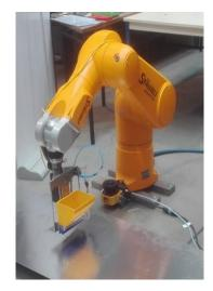
Fig. 4. Staubli TX90 6 axis robot with the sand deposition tool
