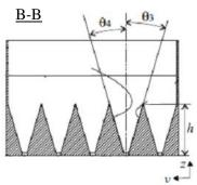
Fig. 22. Inner hopper geometry
