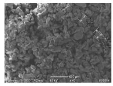
Fig. 20. SEM capture of SiO<sub>2</sub> sand
