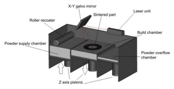
Fig. 1. Double chamber design with overflow bin [9]
